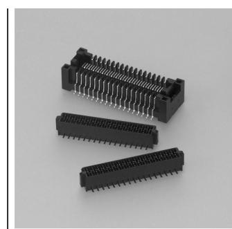
This 0.8mm pitch connector is developed for the car audio industry and is able to compensate for misalignment of up to 0.5mm on all three directions of X, Y and Z axes between the plug and receptacle when they are mating.
